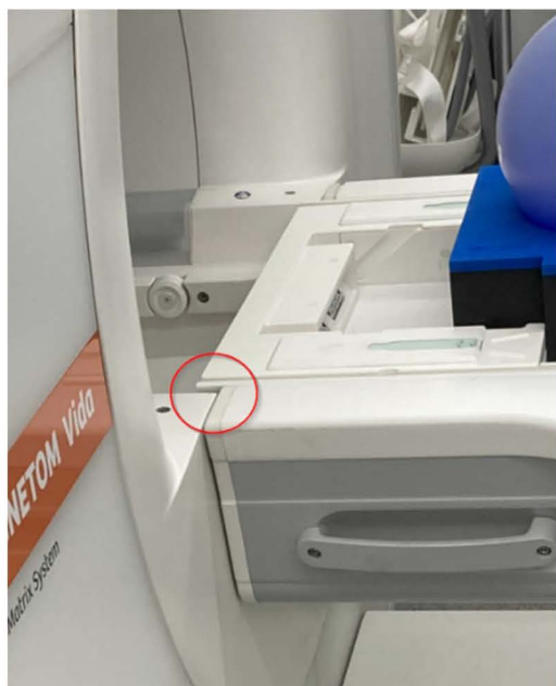
Figure 2: Tabletop moved to home position - Home position with deviation
